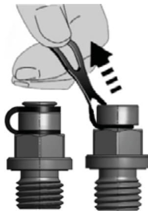
Fig. 6.1.1 Activation of breather plug
