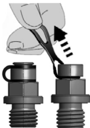
Fig. 6.1.1 Activation of breather plug
