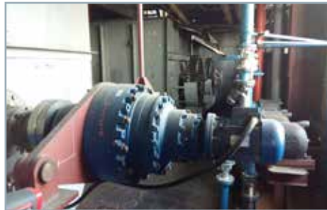
Horizontal crystallizer Planetary EP series
