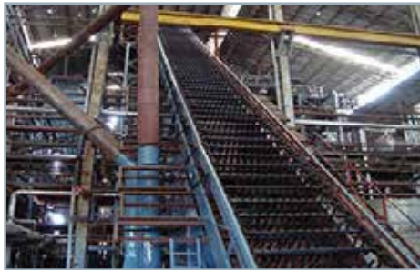
Sugar cane bagasse carrier Helical and bevel helical G and H, planetary EP
