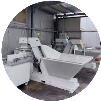
Automatic system for centrifugation of shavings and oil recovery
